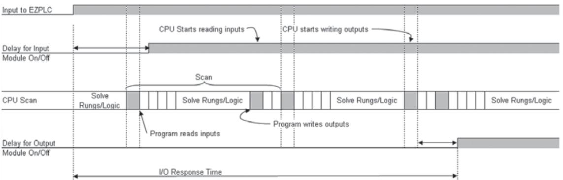
The I/O response time is maximum when the I/O module notes an input change after the Read Inputs portion of the Ladder execution scan cycle. In this case the input status gets noted only in the following Input scan. The diagram shows an example of I/O response timing for this condition. The total I/O response time is calculated as:
