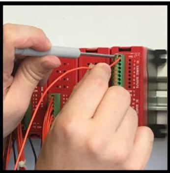
EZRack PLC I/O come standard with spring loaded terminal blocks to provide a secure connection and easy field wiring experience.
