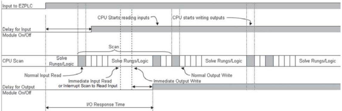
Using Interrupt subroutines and Immediate I/O instructions is the best way to optimize the I/O Response time of your EZRack PLC system. The immediate instructions update the I/O points during the ladder logic program execution.
