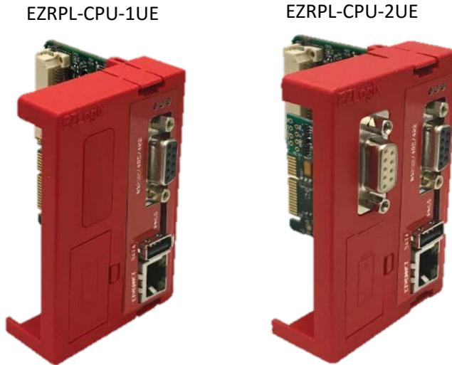
EZRack PLC has two different CPU options. It comes with either 1 or 2 serial ports built on it.
