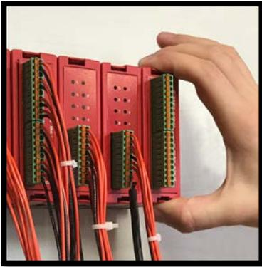
EZRack PLC I/O modules have a snap on design to facilitate easy installation and removal from base slots. The I/O modules have 2 clips, one on the top and the other on the bottom and a connector on it's base, which plugs in to the EZRack PLC base through the guiding slot.
