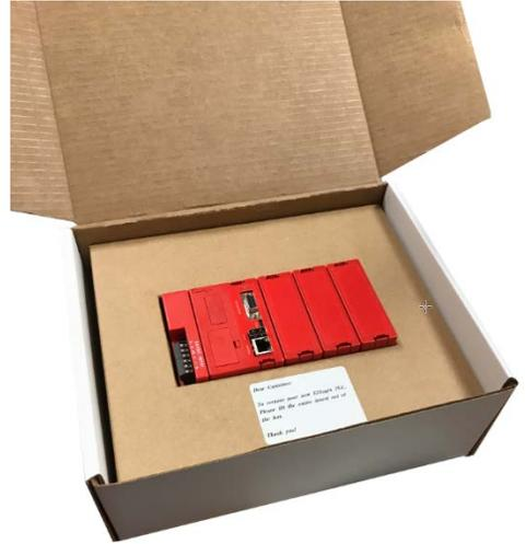
**Step 2:** Remove any blank modules by pressing on the top and bottom tabs and pulling out from the base. Replace blank module with one of the EZRack PLC I/O modules. When inserting the EZRack PLC I/O module make sure to line up the module on the “guiding slot” and press firmly till it snaps to the PLC base.
