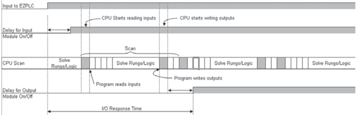
See the diagram above. The I/O response time is minimum when the I/O module gets the input change before the Read Inputs portion of the Ladder execution scan cycle. In this case the input status is read, the logic program is solved, and the corresponding output point gets updated. The total I/O response time is calculated as:
